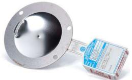
The LOTRX® Rupture Disc is a scored reverse acting rupture disc that utilizes a failure initiating indent, a highly accurate manufacturing method to achieve and control a burst pressure at close tolerances, plus a precision semicircular score to provide a clean, consistent opening pattern.
