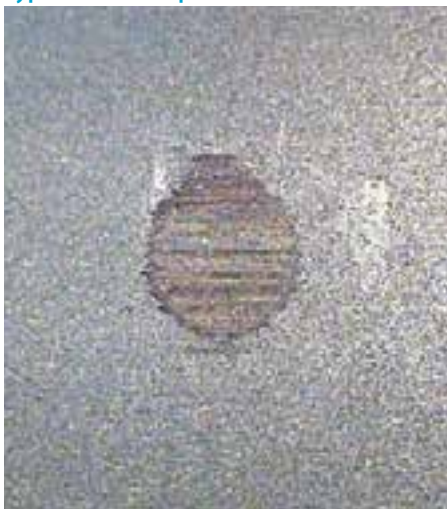
Figure 4 Typical wear dimple after 15 min
