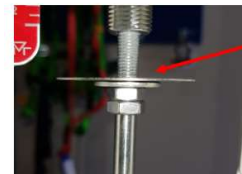
Travel Indicator, washer & valve stem locknuts.
