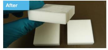
The images above show the foam samples before and after the test; as one can see the samples look as good as new, even after 28-days exposure to a variety of fungal spores in high humidity.
