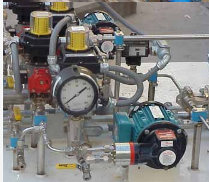
Hydra-Cell (30kgs) is compact compared to traditional metering pumps (100kgs)
