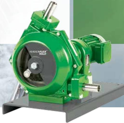
The Verderflex Rollit is a series of easy to use, lubricant free hose pumps for flow rate up to 24.5 m<sup>3</sup>/h. Easy to maintain, with 3 rollers for less pulsation. Energy efficient Verderflex Rollit pumps are dry self-priming up to 8 mwc and are available as single and twin channel models.
