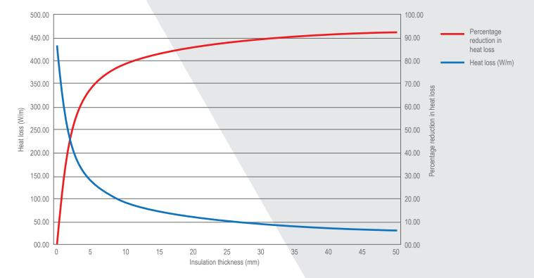
This would suggest that it is more important to ensure maximum coverage of pipework with insulation than it is to insulate easy-to-reach portions of piping with very thick insulation, leaving some pipework bare.
