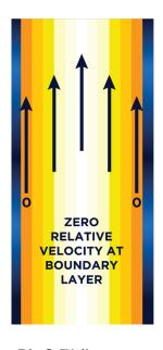
Discflo™ disc pumps employ the principles of Boundary Layer and Viscous Drag, to produce pulsation-free laminar flow. Typical pipe flow showing Boundary Layer and Viscous Drag Hydraulic Principles.
