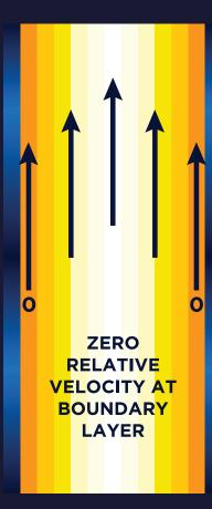
With no impingement device to damage your product and a boundary layer of protection for the pump, the Disc pump effectively eliminates the root cause
